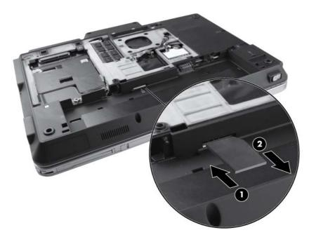
Reverse this procedure to install the SIM.
